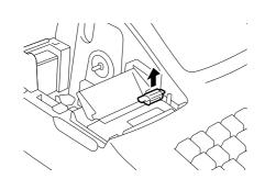
Pinch the Ink Roller Knob with your fingers, and pull it upward.
